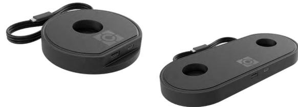
*D1UB-NA Single and D2UB-NA Dual Charging Hub*
