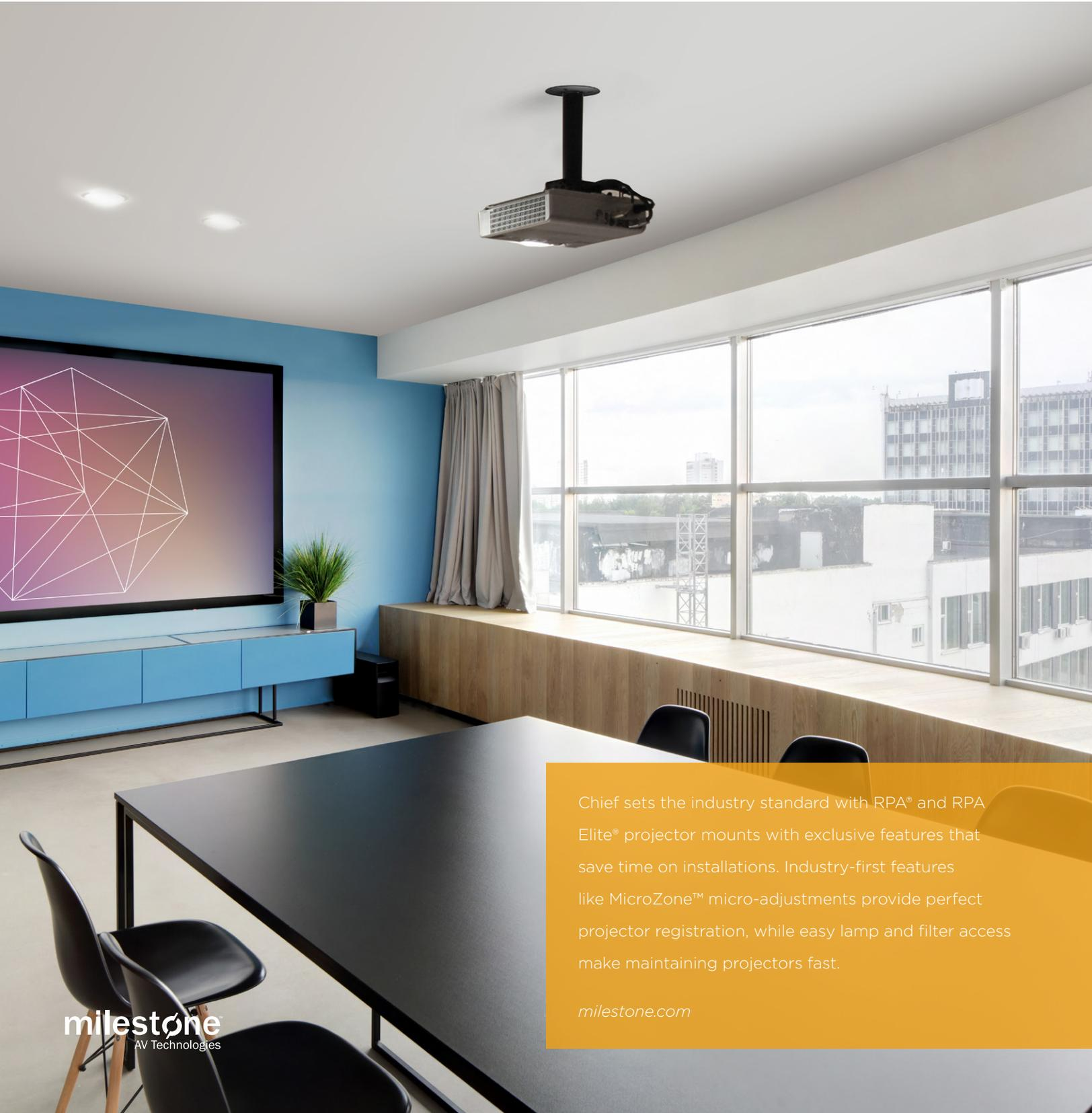
Chief sets the industry standard with RPA® and RPA Elite® projector mounts with exclusive features that save time on installations. Industry-first features like MicroZone™ micro-adjustments provide perfect projector registration, while easy lamp and filter access make maintaining projectors fast.
