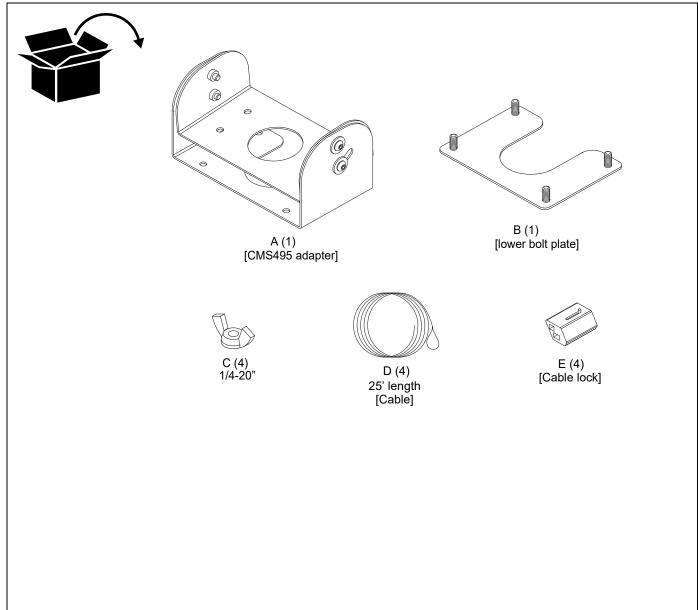
**IMPORTANT !** : The CMS495 was designed specifically to be used with the UL Listed CMS440 Lightweight Suspended Ceiling Kit in order to make it compatible with ceilings angled up to 45°. Do NOT attempt to use the CMS495 with any other type of ceiling mount!
