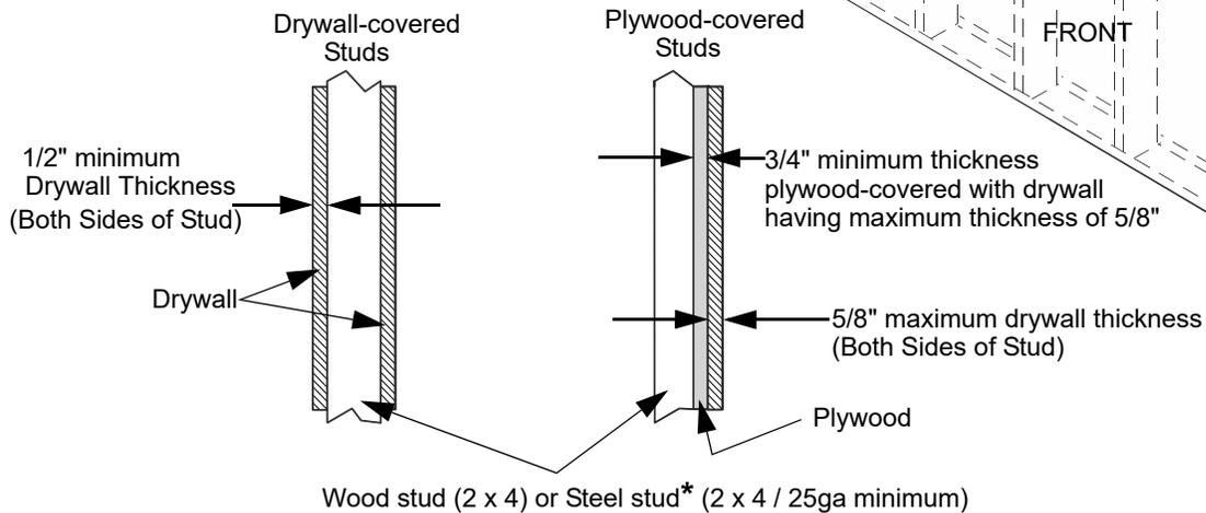
\*Steel stud type and structural strength must conform to the North American Specification for the Design of Cold-Formed Steel Structural Members. [362 S 125 18, C-Shaped, S-Stud Section]
