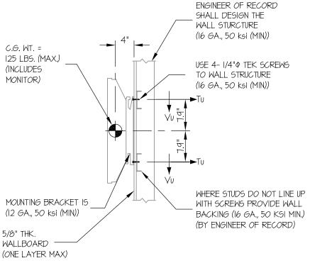
Tu = 77 LB/SCREW (MAX) Vu = 67 LB/SCREW (MAX) SIDE ELEVATION AT STEEL STUD WALL
