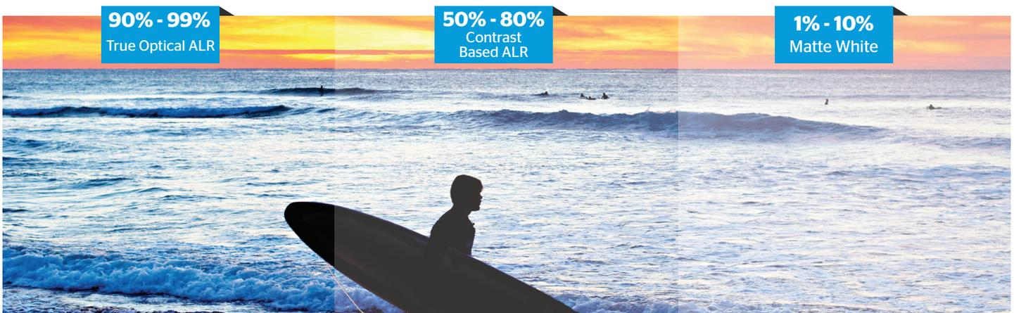
Side by side illustration of Ambient Light Rejection surfaces; True Optical ALR screens provide the best image contrast, color saturation and dynamic range.
