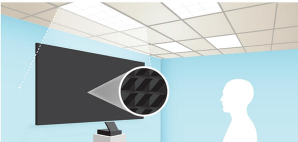
Illustrations of the microscopic saw-tooth layer that blocks light from above in True Optical ALR surfaces.
