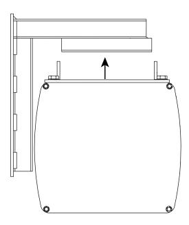
4. When the sliding bracket on the case and the wall bracket allign, take the security bolt (C) and screw in place.
