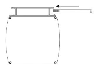
5. Tighten the security bolt on all 3 brackets until the case is fully secured.
