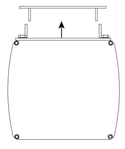
4. When the sliding bracket on the case and the ceiling bracket allign, take the security bolt (B) and screw in place.
