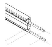
8.2 Screens wider than 400 cm require a spreader bar. Connect the top and bottom frame with the spreader bar and connect this by using the two supplied screws (D).
