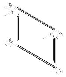
1. Unwrap the frame pieces. Before assembling the frame pieces, add 2 nuts (A) to either end of the top frame section and the top of the side frame for the mounting bracket and add 2 nuts to the bottom frame.
