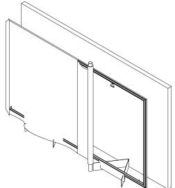
10. First tension the surface so the end of the surface alligns with the frame end. After the entire screen is attached, you can adjust tensioning where necessary.
