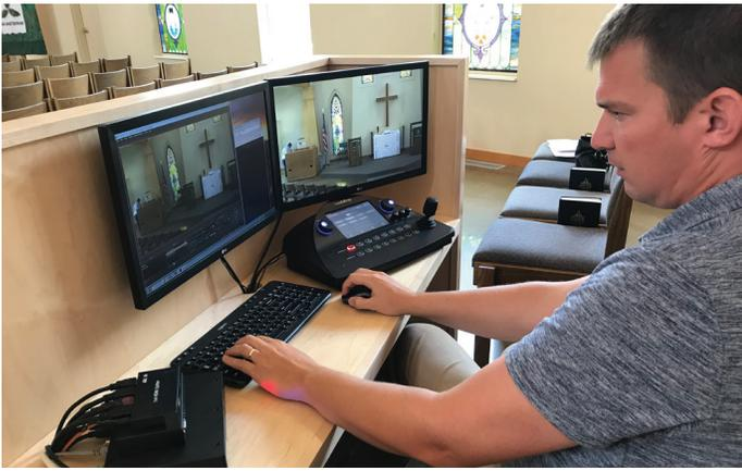
The OneLINK Bridge mixes the in-room audio with the RoboSHOT video into a single USB stream onto the computer where they can stream and archive the service to YouTube. The OneLINK Bridge also keeps them from having to use a daunting sound mixer. Instead, they can use the web interface to adjust volumes of the audio inputs and have a matched video/audio feed to send wherever they need it. The OneLINK Bridge uses a single cable to provide power, video and control to the camera.
