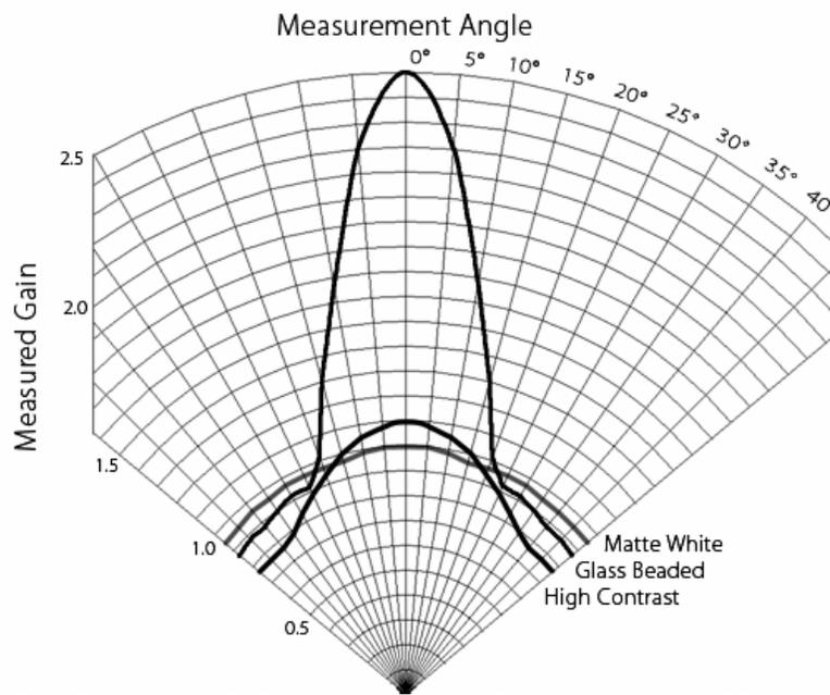
*Figure 2 – Gain measurements of three screen materials plotted around a central point to represent the measurement angles more directly*
