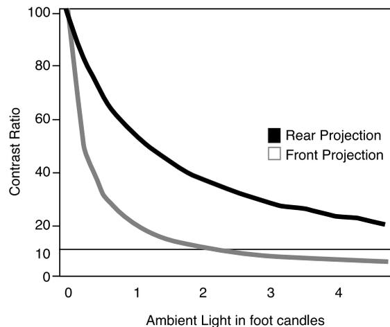
From Angles of View Volume V, we also learned that we should design systems such that the contrast ratio should be at least 10:1. All right, that is all well and good but how do we determine this? First we must look at the equation we were given from this article. It states the following:
