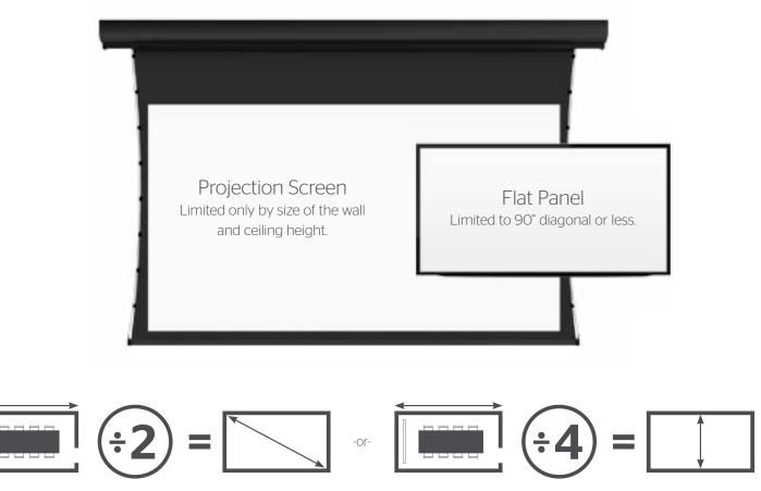
**For 16:9 and 16:10 Formats:** An easy way to determine screen size is to take the depth of the room and divide by two. This will equal the approximate diagonal of viewing area for your audience in 16:9 or 16:10 format.
