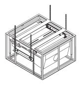
Method A **Unit Attached To Threaded Studs**
