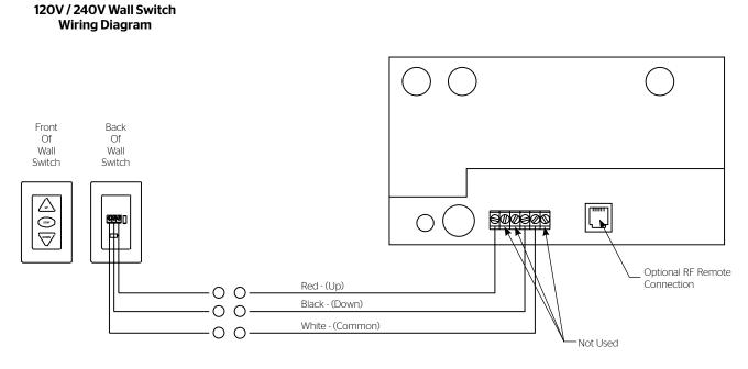
**NOTE:** 20-24AWG wire recommended for connecting wall switch to sychronization controller.
