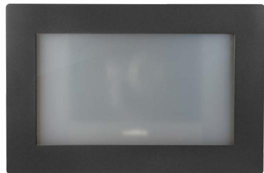
*Equipped with laminated safety glass, Vaddio RoboSHOT IW Smart Glass PTZ Camera changes from frosted opaque when the camera is off to a transparent clear glass when the camera is powered on.*
